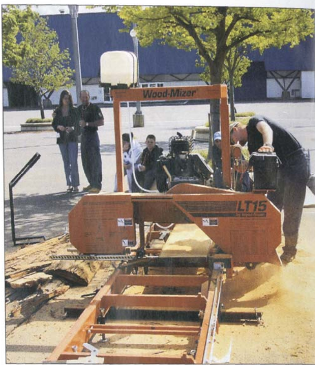
Thin kerf sawmills can allow more usable lumber to be recovered from a typical log, an especially important virtue when cutting irreplaceable woods with historic or personal value.
